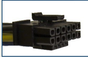
12+4-Pin PCIe 12VHPWR Cable
